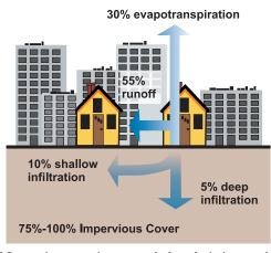
Relationship between impervious cover and surface runoff. Impervious cover in a watershed results in increased surface runnoff. As little as 10 percent impervious cover in a watershed can result in stream degradation.
